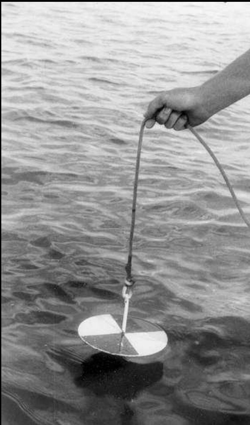
**Secchi disk (SD) about to be lowered into water. SD depth is the greatest depth (measured in metres) at which disk pattern can be visualized**
